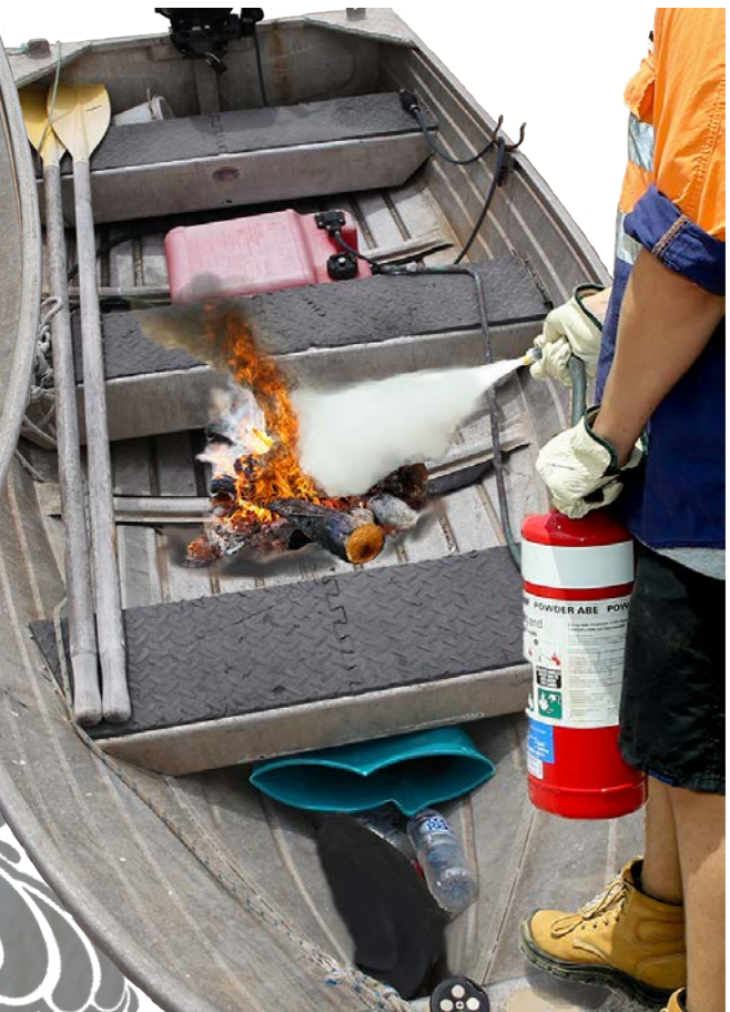
Using a fire extinguisher on a boat fire
