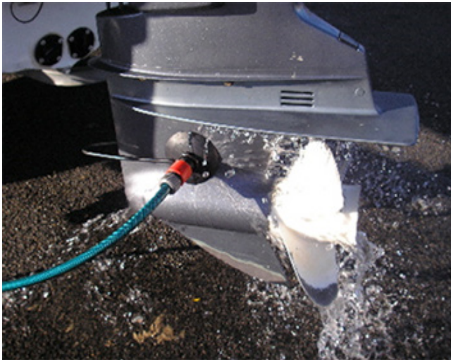
Flush the outboard motor
