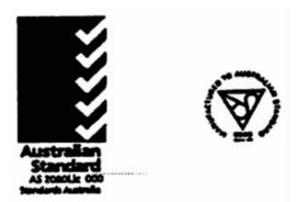
The glass must always bear an identification mark indicating the standard to which the glass has been manufactured (e.g. AS2080, BSAU178, JISR3211, ECER-43/00, ANSI-Z26.1) and have a standards mark etched or indelibly printed on the glass.
