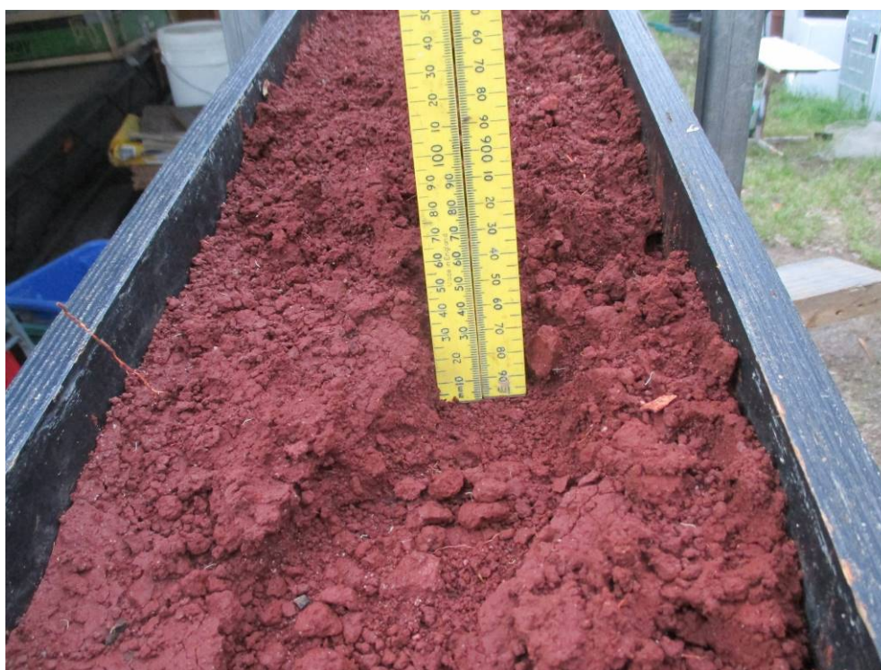
Figure 10. Eroded surface at the end of the 15% run for NPT01 0.5m-1.1m (Red) material.
