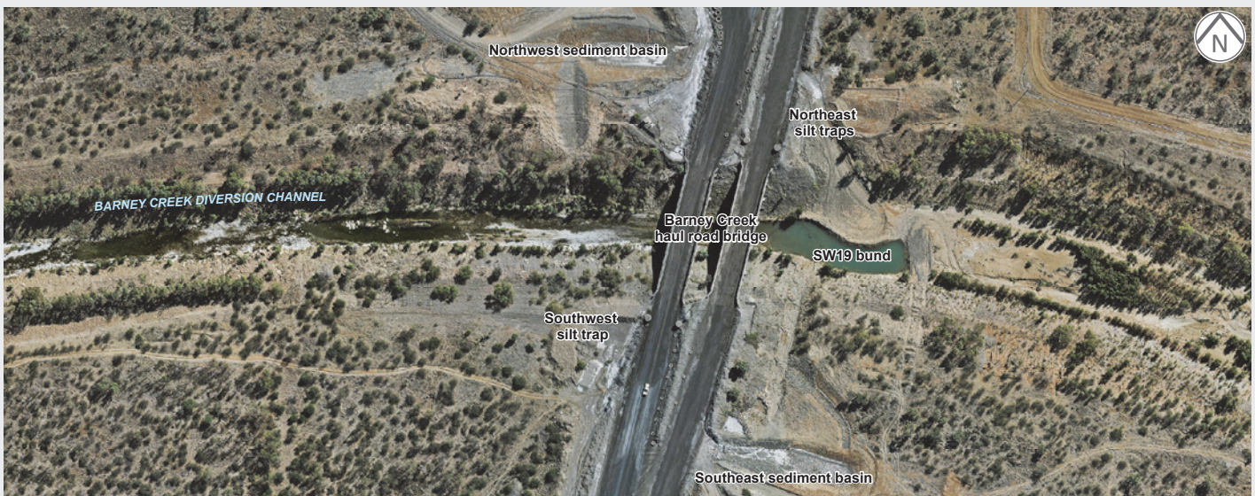
Sediment control structures at Barney Creek haul road bridge
