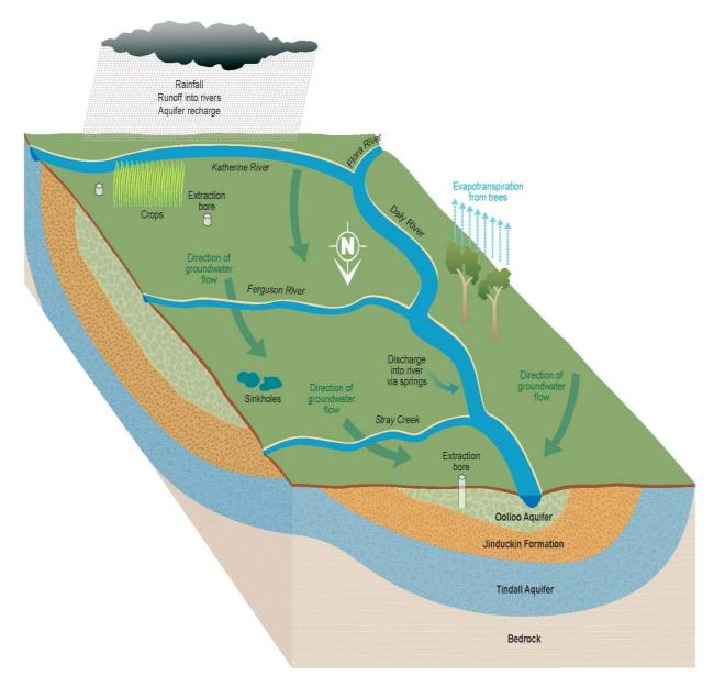
Figure 3 Conceptual diagram of the Oolloo Dolostone Aquifer
