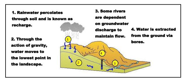
Figure 2 Conceptual Groundwater Diagram
