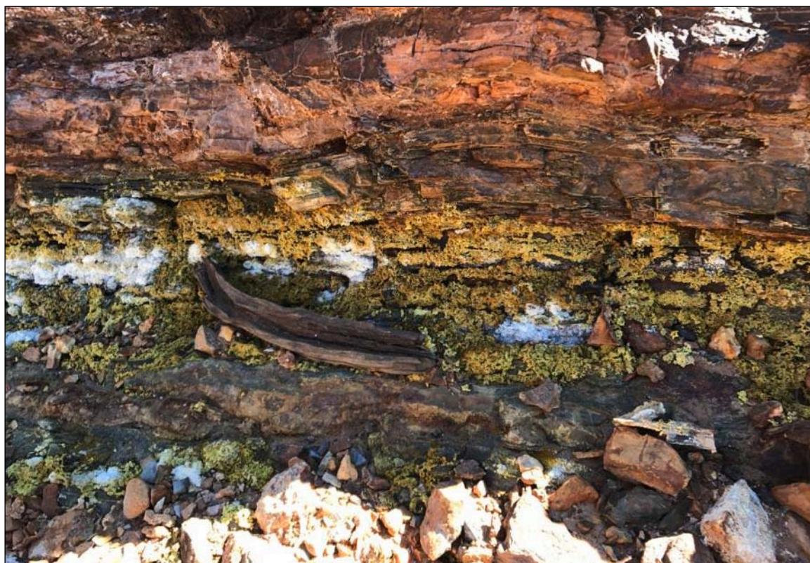
Plate 4.10 – Intense Salt Crusting on Pyritic Units Exposed in the McArthur River Diversion Channel Between SW15 and SW16
