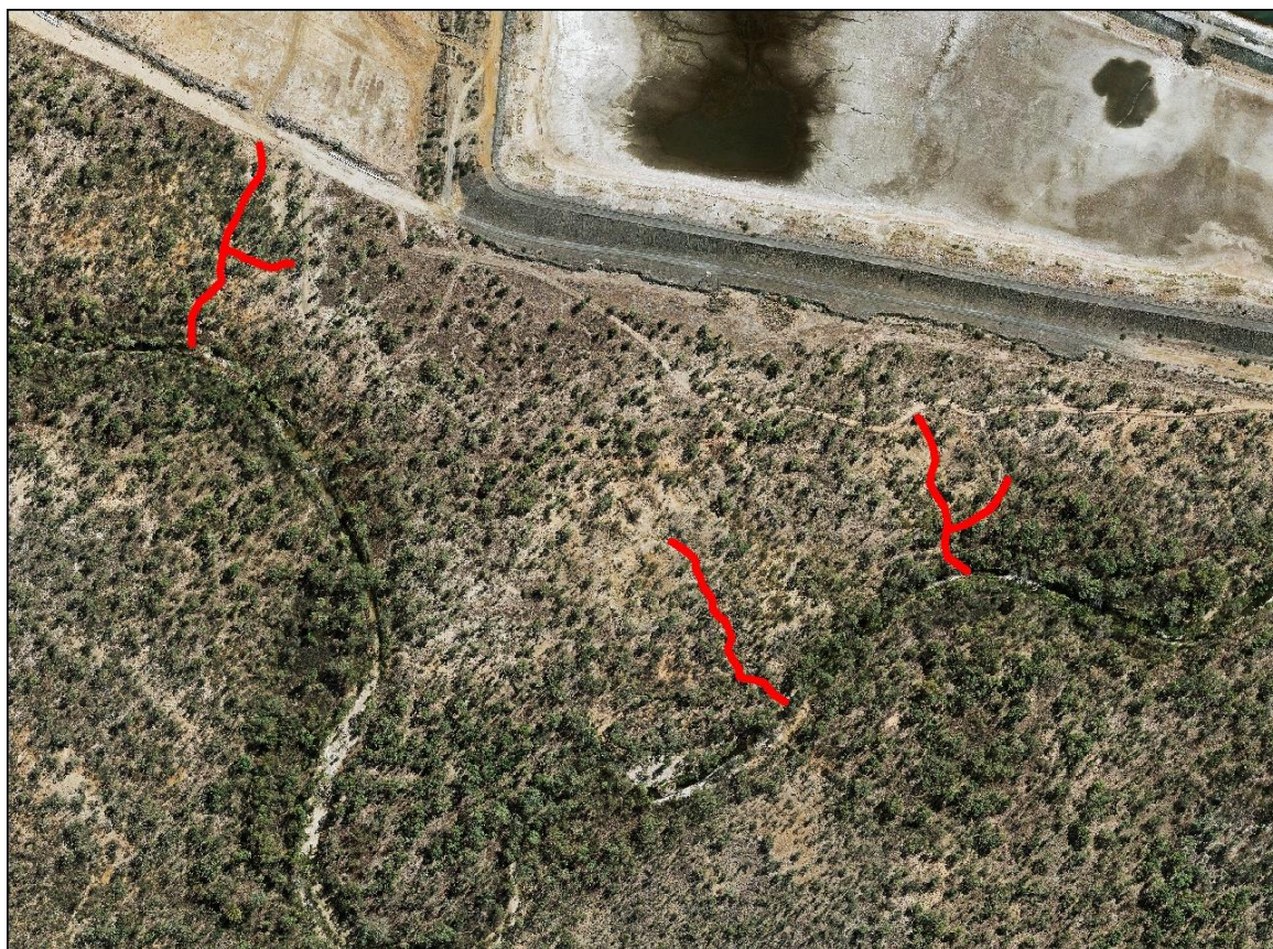
Plate 4.1 – Location of Erosion Gullies on Surprise Creek Southwest of the NOEF SPROD
