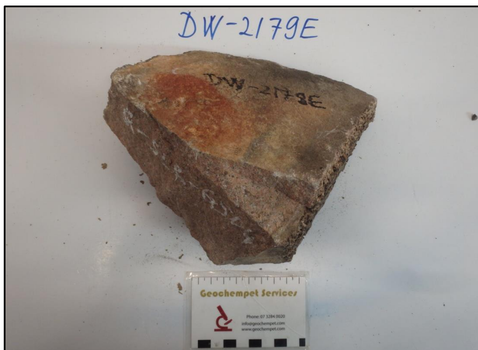
Figure 1: Photograph of washed sub-sample from supplied aggregate
