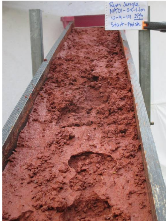
Figure 10. Eroded surface at the end of the 15% run for NPT01 0.5m-1.1m (Red) material.
