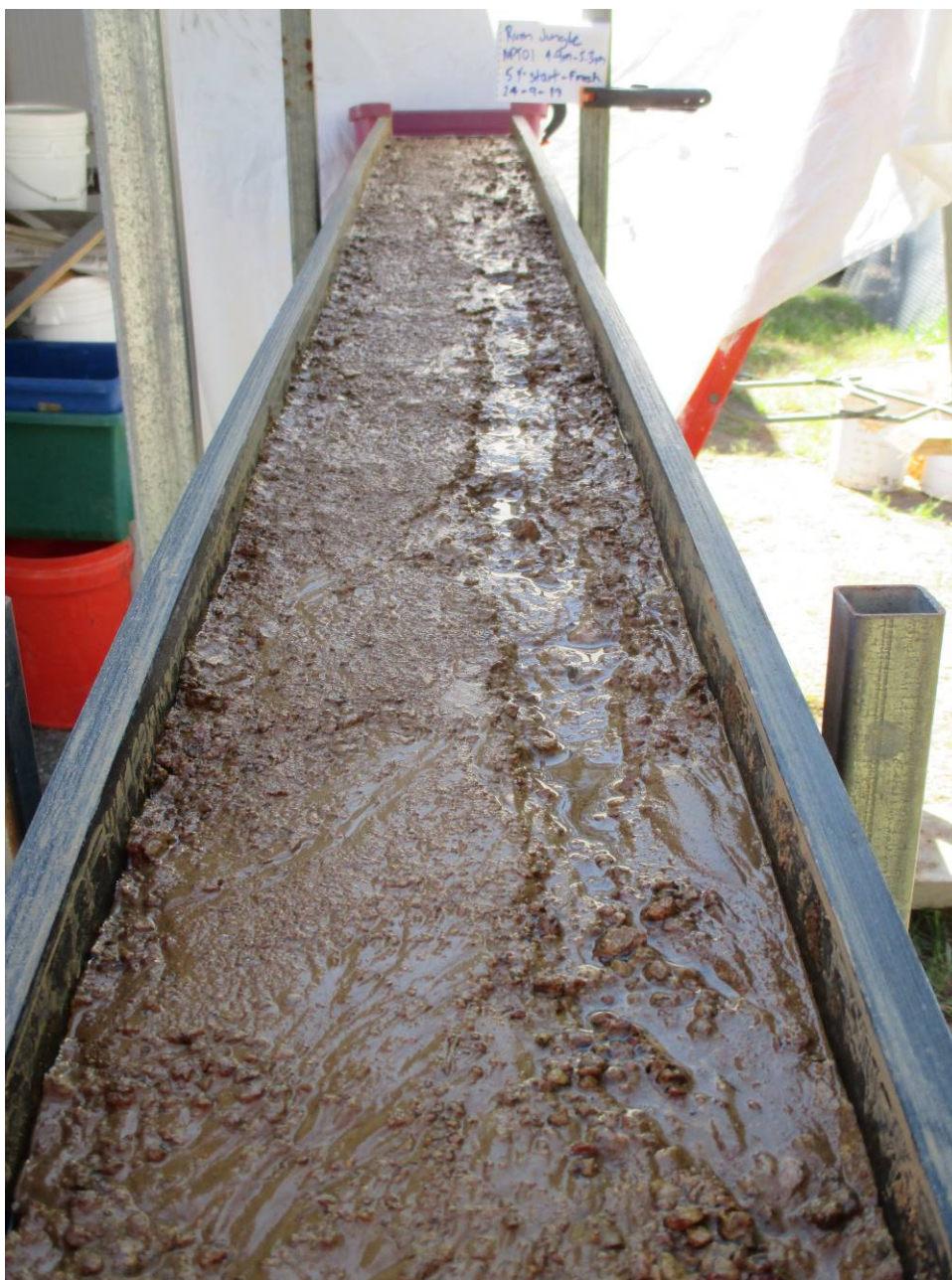
Figure 14. NPT01 4.9m-5.3m (Tan) 5% slope at the end run. Note the rill running the length of the flume.
