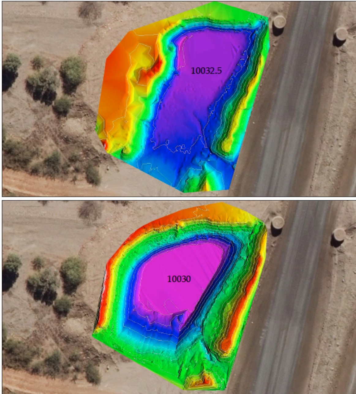
Plate 4.13 – Upgrades to Haul Road Bridge Southwest Sump (Before/After)
