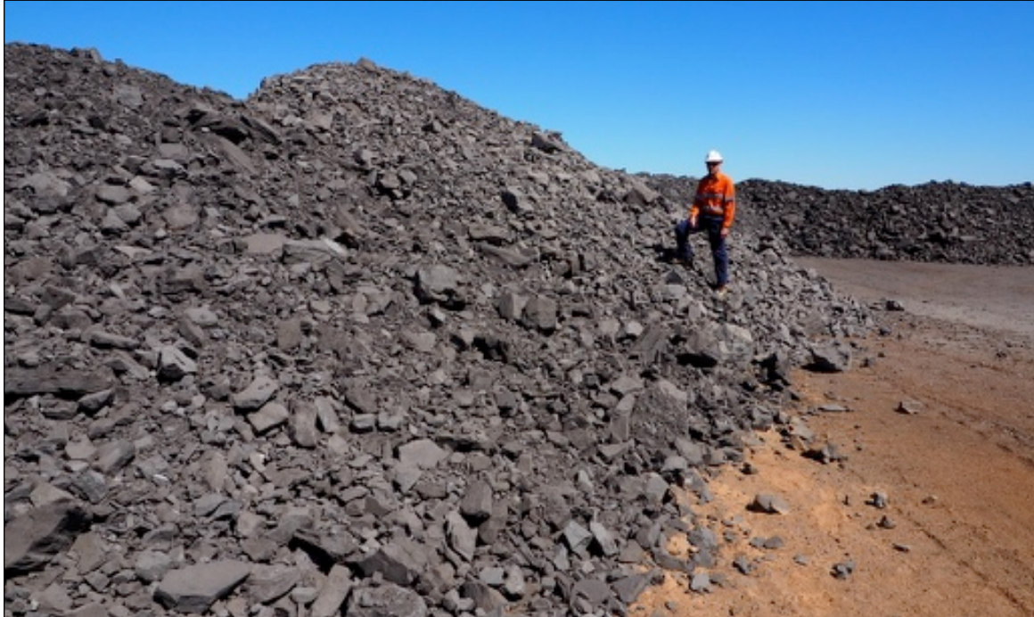
Plate 4.2 – End-tipped PAF Profile in the CW Stage of the NOEF
