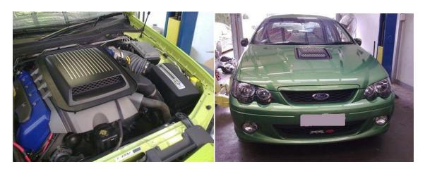
A scoop that is affixed to the engine itself (i.e. "GT Shaker style") may be acceptable provided it meets the general requirements applying to bonnet scoops and external protrusions as out lined in ADR 42/--- or ADR 92/--- with the additional requirements:
