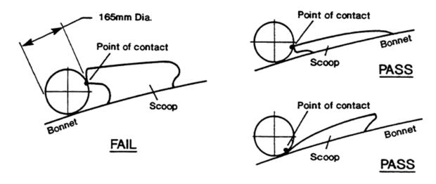
• The driver must be able to see the surface of the road 11m in front or all of the front edge of the original body when looking across the top of the scoop. For the purposes of this requirement, the driver's 'eye' position can be taken as being a point 730mm above and 270mm forward of the junction of the seat cushion and seat back with the seat in its lowest and rearmost position.
