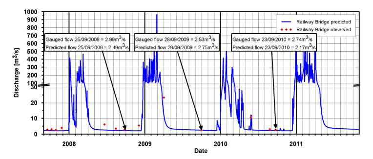
Figure 1: Observed and predicted discharge of the Katherine River at the Railway Bridge from mid 2007 to mid 2011.
