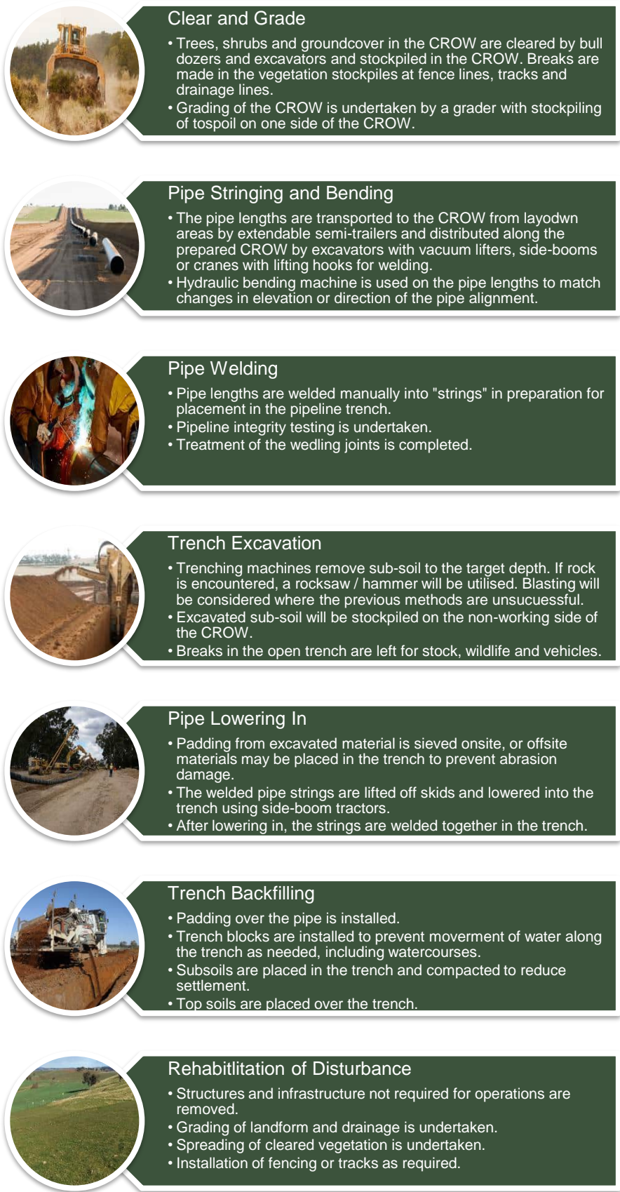
Figure 9: Stages of Trenched Pipeline Construction
