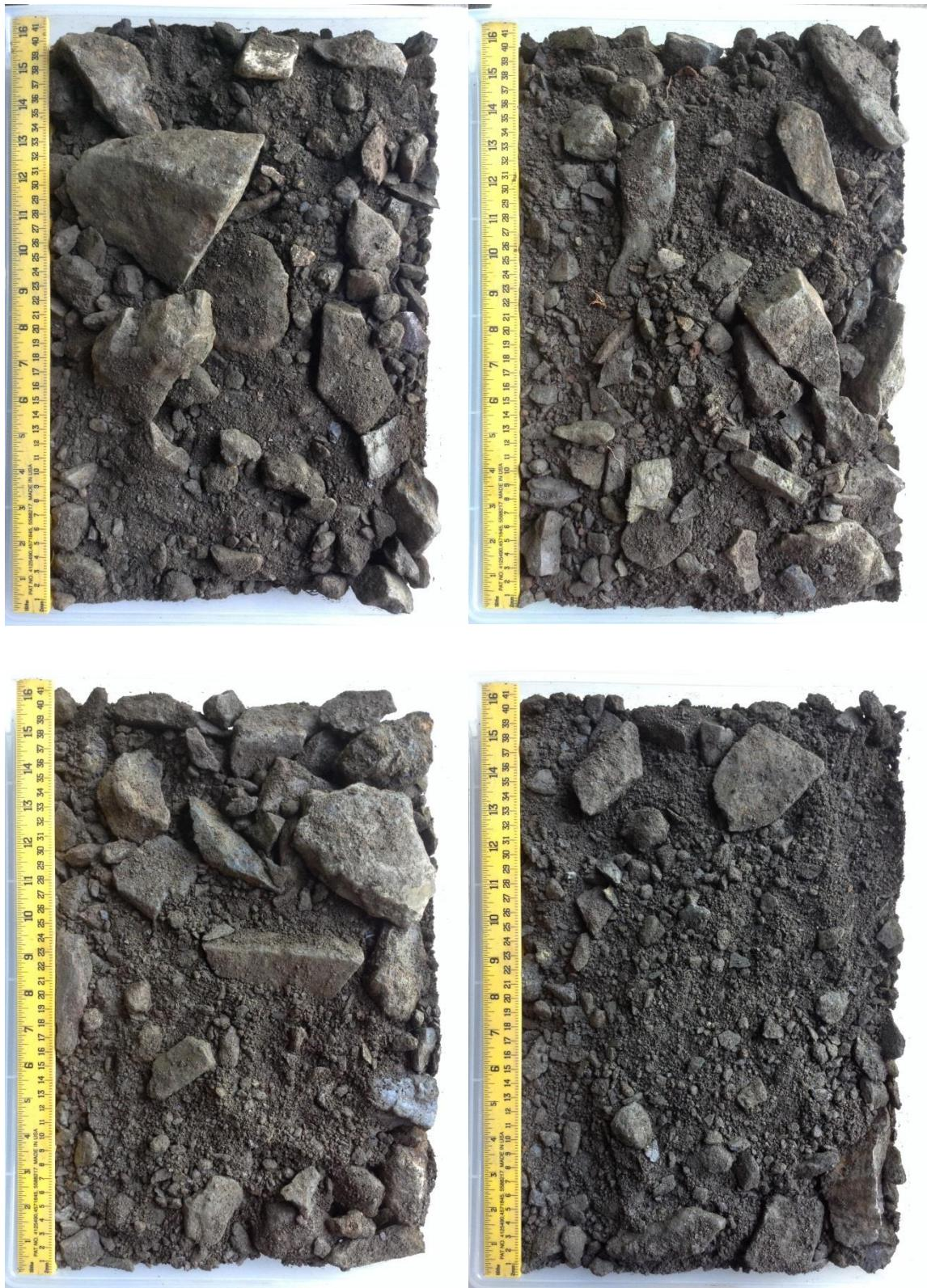
**Photo C1 18: TP3-P2 waste rock samples from depths a) 1 to 2 m; b) 2 to 3 m; c) 3 to 4 m; d) 4 to 5 m**
