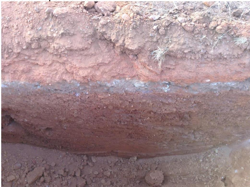
**Photo B8 19: TP49 test pit (left); waste rock samples collected from 0.55 to 0.80 m (right)**
