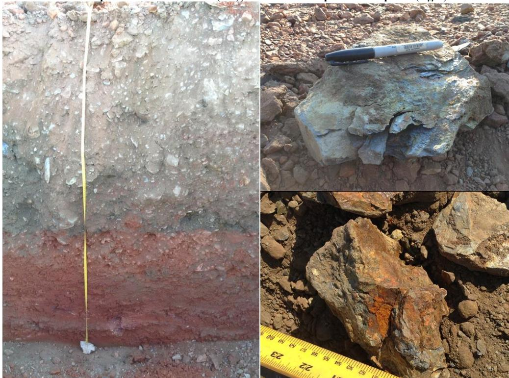
**Photo B8 11: TP45 profile from 0 to 2.0 m (left); close up of top 0.7 m (right)**
