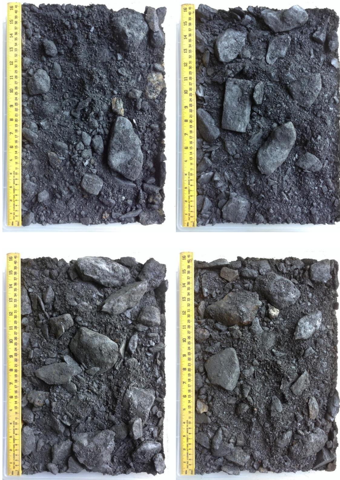
**Photo C2 2: TP4-P1 waste rock samples from depths a) 5 to 6 m; b) 6 to 7 m; c) 7 to 8 m; d) 8 to 9 m**
