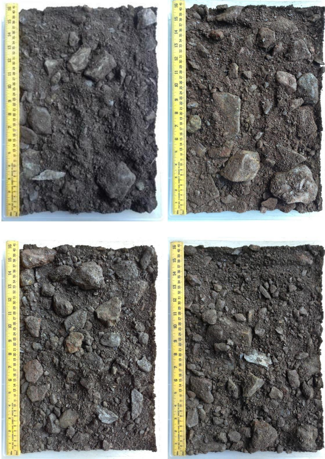
**Photo C1 4: TP1-P1 waste rock samples from depths a) 13 to 14 m; b) 14 to 15 m; c) 15 to 16 m; d) 16 to 17 m**
