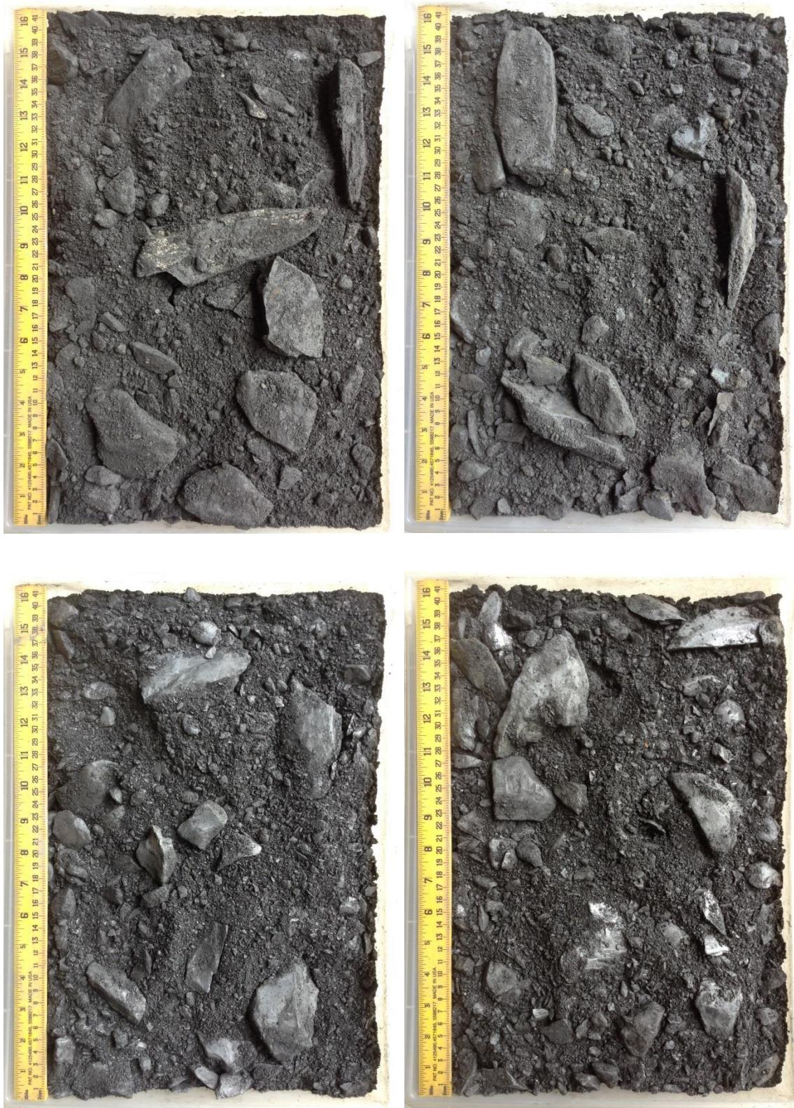
**Photo C2 9: TP7-P1 waste rock samples from depths a) 4 to 5 m; b) 5 to 6 m; c) 6 to 7 m; d) 7 to 8 m**
