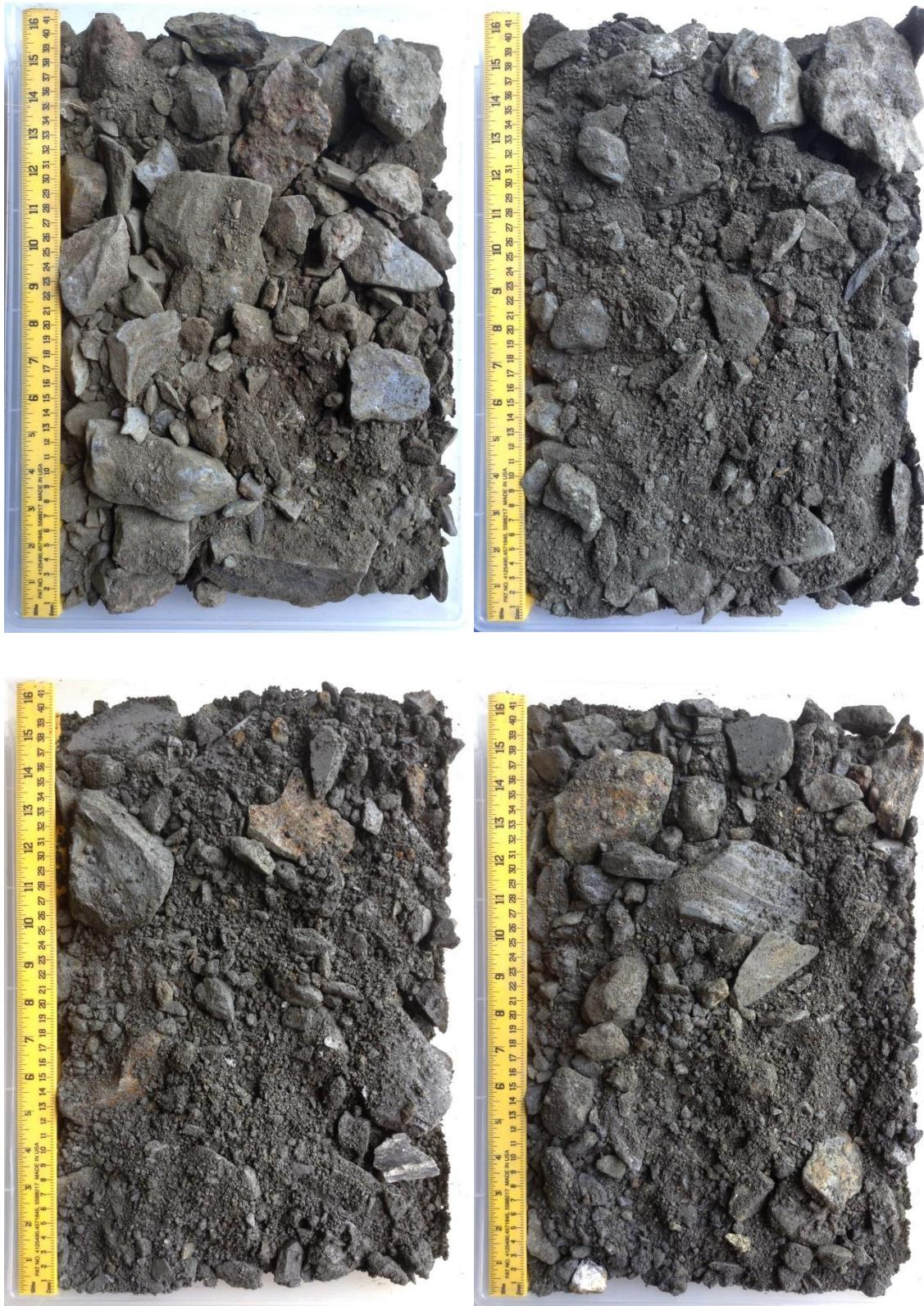
**Photo C1 11: TP2-P1 waste rock samples from depths a) 4 to 5 m; b) 5 to 6 m; c) 6 to 7 m; d) 7 to 8 m**
