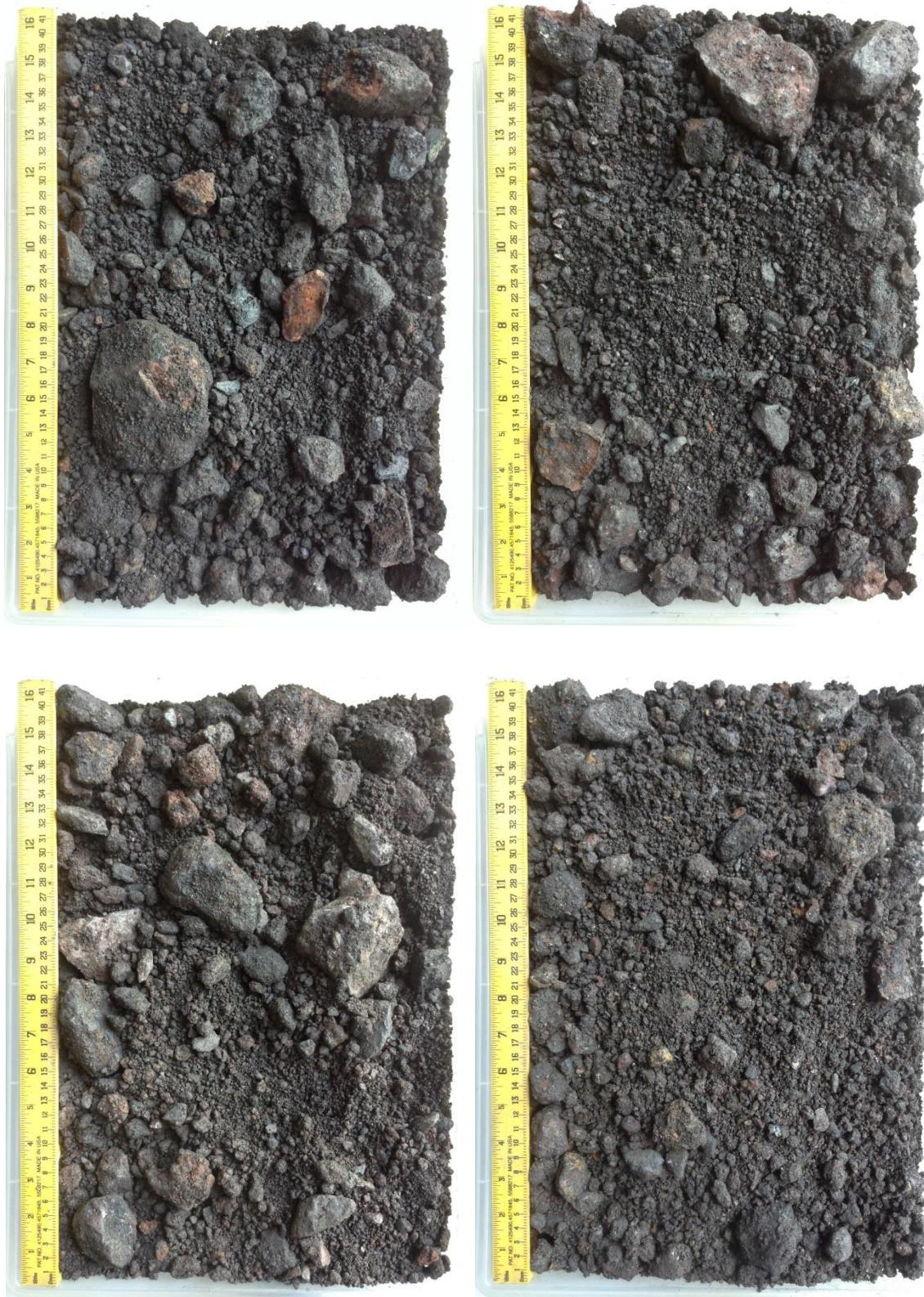
**Photo C3 2: TP6-P1 waste rock samples from depths a) 5 to 6 m; b) 6 to 7 m; c) 7 to 8 m; d) 8 to 9 m**
