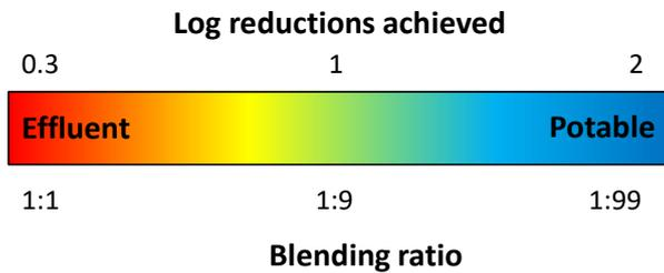
The quality of the water the effluent is blended with affects the achievable LRV. Storm water which may be contaminated from runoff will require a greater blending volume or depending on its water quality, may result in a pathogen increase in the blended water. The illustration below shows the actual log reductions achieved when effluent requiring 3 LRs is blended with stormwater requiring 1.5 LRs for the end use.
