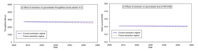
Figure 9 predicted effects of extraction scenarios on a) throughflow to the north and b) water levels at RN12395.
