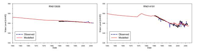
Figure 5 Comparison of the predicted and observed groundwater levels in the vicinity of the Table Grape Growers of Australia borefield.
