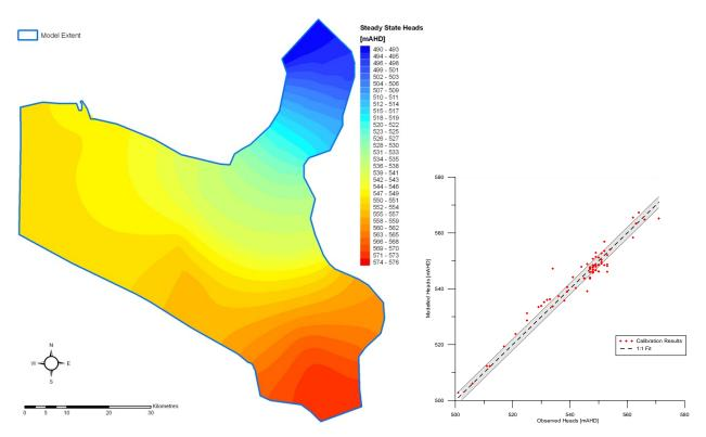
Figure 2 Steady state calibrated heads. The envelope along the 1:1 fit identifies the expected error in measured observations.
