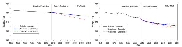
Figure 8 Predicted water levels in response to pumping at TGGA a) RN13926 and b) RN14191.
