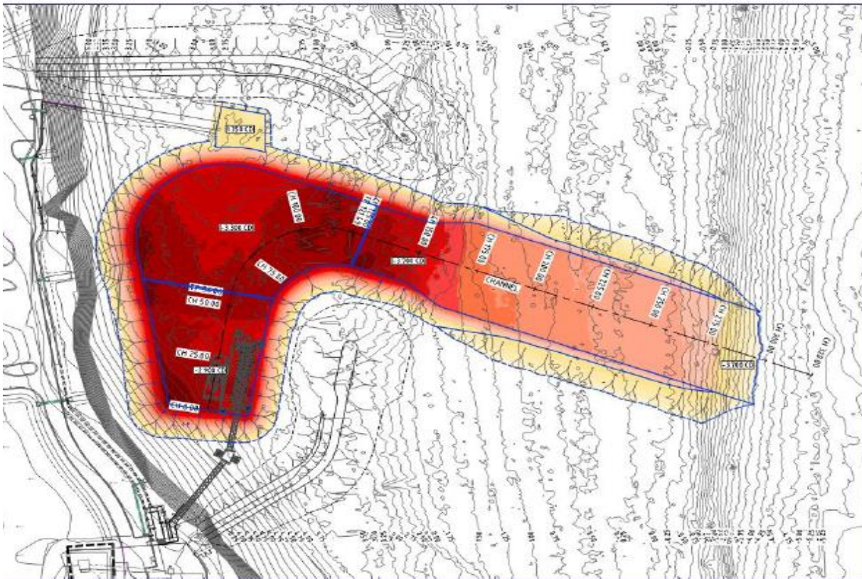
Figure 2: Dredge excavation profile
