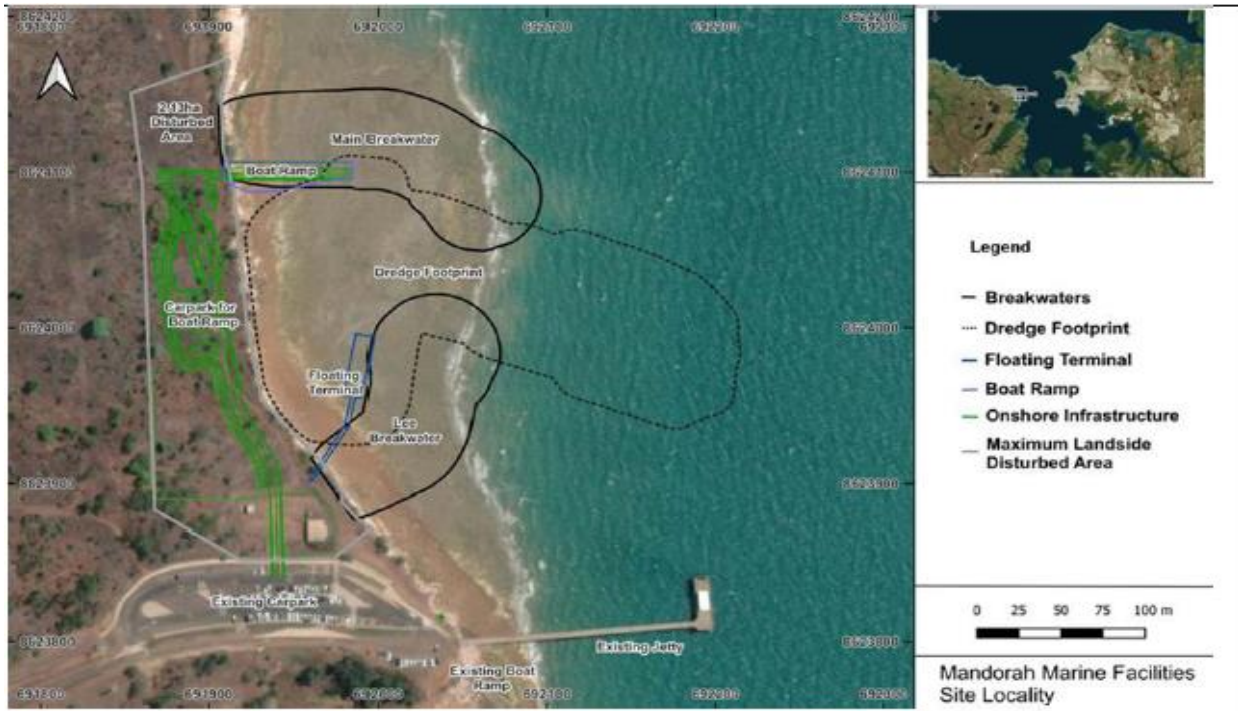
Figure 1: Dredge and breakwaters in proximity to existing Mandorah jetty.
