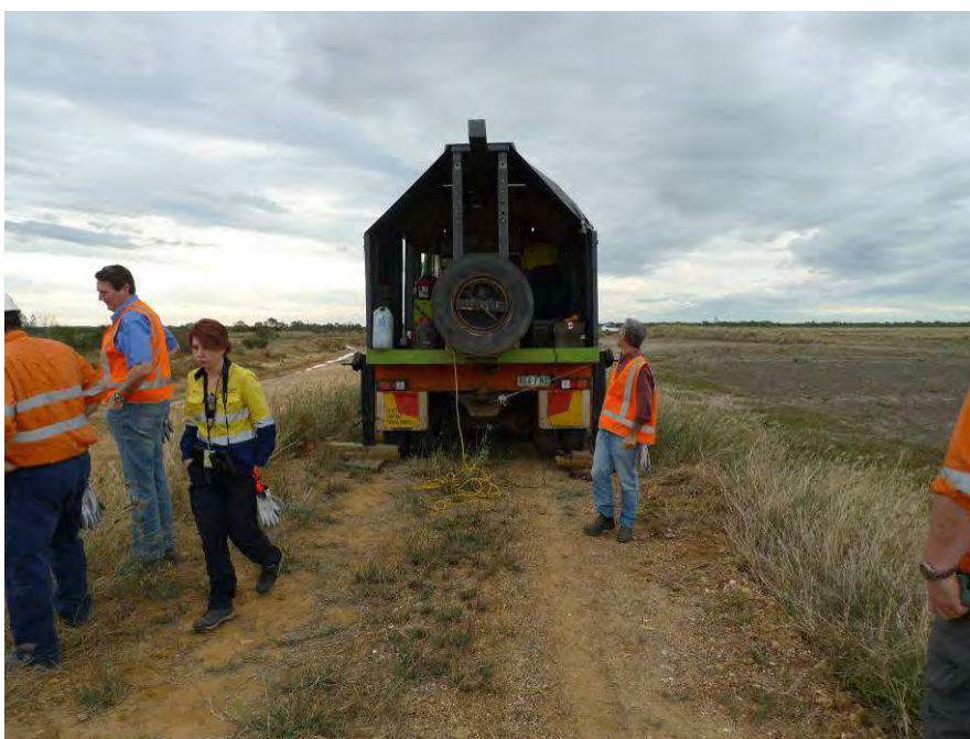
Plate 41 Cone Penetrating Testing (CPT) geotechnical investigation being undertaken on the Bing Bong dredge spoil walls during the Independent Monitor's May 2012 site inspection.
