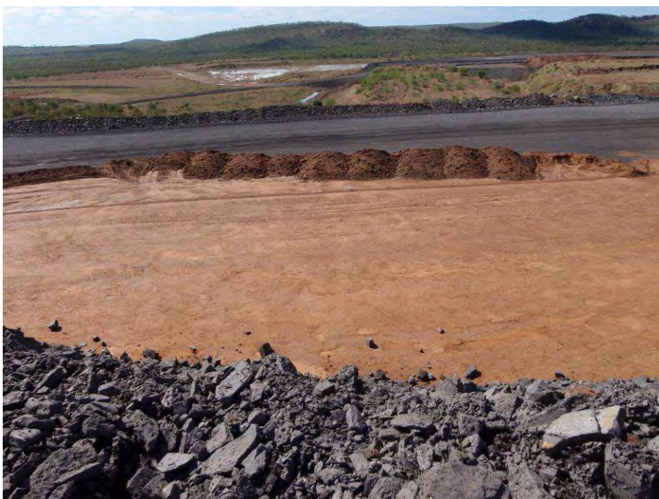
Plate 38 Area of exposed clay liner has been reduced when compared to previous years, which is a positive improvement.
