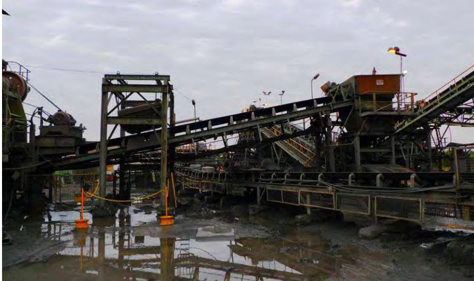
Plate 5 PACRIM crushing plant located on the ROM Pad at the mine site. Note the area is kept moist with sprays on the conveyor belts to limit dust generations.
