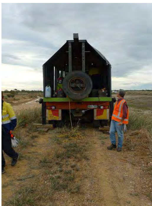
Plate 3 Bing Bong surface water management improvements: a) geotechnical testing of the Bing Bong dredge spoil walls to gain an understanding of the material makeup of the walls, and thus, the potential for saline seepage through the walls; and b) tanks have been installed around the Bing Bong concentrate storage shed to capture clean rain water and divert it to sea, rather than to onsite storage during the Wet Season.
