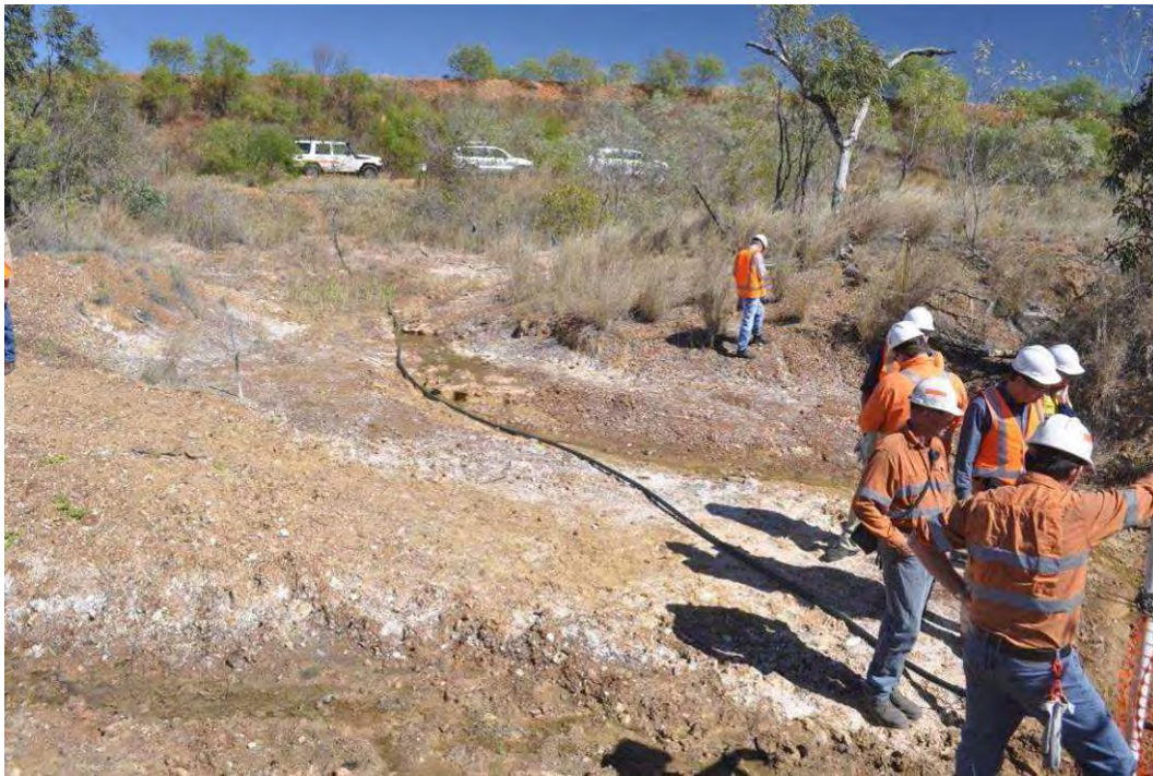
Plate 21 Salt accumulation from tailings seepage at Surprise Creek observed during May 2012. The water quality of seepage appeared to improved since the previous year, perhaps due to reduced water levels in the TSF or from fresher water travelling subsurface from the WMD.
