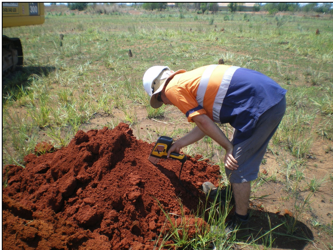
Figure 4. Hand Held FPXRF analysis of soil in Zone 2 (2)
