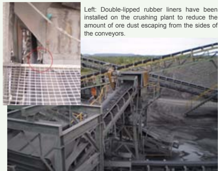
The ore crushing plant that operates on the mine site is a source of ore dust-generation, which can contaminate soil and water. Steps are being taken to limit dust from this facility.
