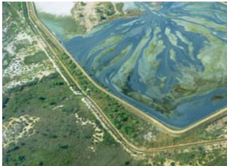
Aerial view of the northern-most Dredge Spoil pond with perimeter spoon drain, and dredged material and sea water radiating from the central deposit point in the middle of the spoil pond (May 2010).
