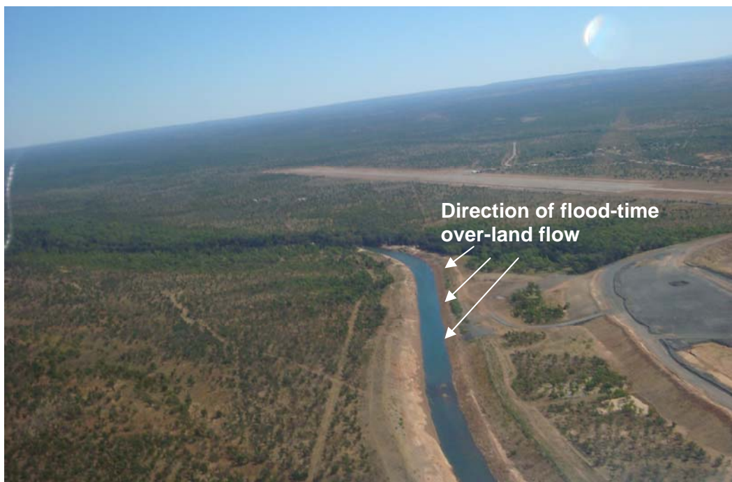
Plate 59 Aerial view of the McArthur River diversion channel showing the direction of the overland flood flow path from the old river channel to the diversion channel. Post 2010/2011 wet season scour was observed at the toe of the mine levy and over the area over which the water passed. Photo: Independent Monitor
