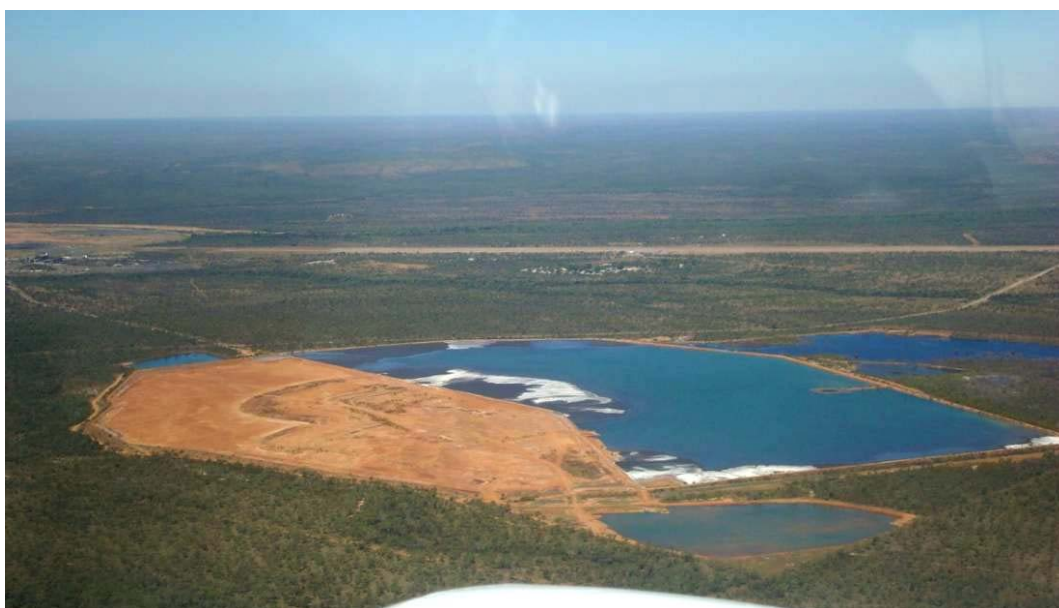
Plate 2 Excess water still stored in TSF Cell 2 in 2011. Note the completion of the clay capping of TSF Cell1 since the previous audit. The cap now acts as a measure to suppress talings dust emissions. Photo: Independent Monitor, 1 June 2011.
