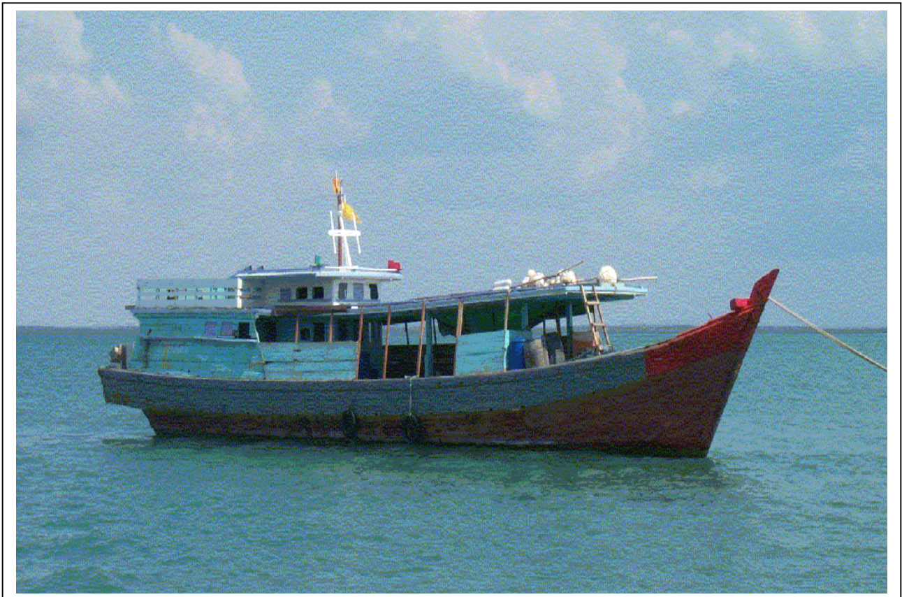
Figure 2. Indonesian type 3 Iceboat from the Province of Probolinggo
