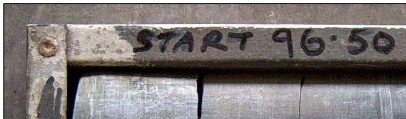
Figure 1 Label the starting depth of the cored interval on the top left corner of the tray
