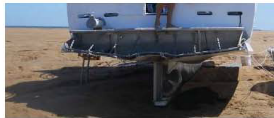
Beached vessel resting on keel without support.
