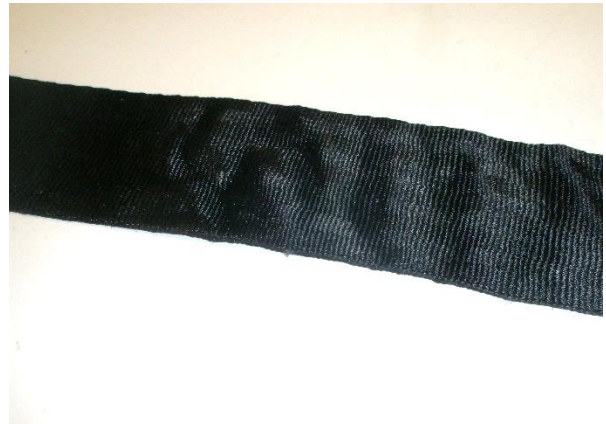
Rippling (crash damage)
