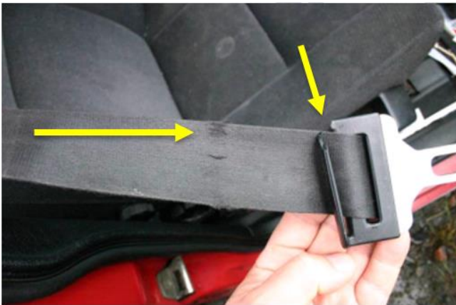
Stretch damage (crash damage)
