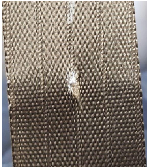
Hole (cut threads)
