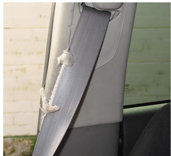
Fraying (outer weave compromised)
