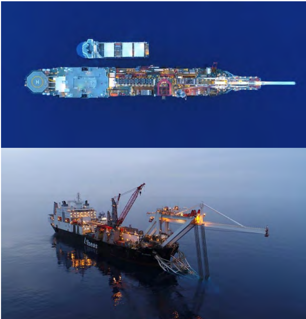
Figure 5-1: Photographs of a typical pipelay vessel at dusk
