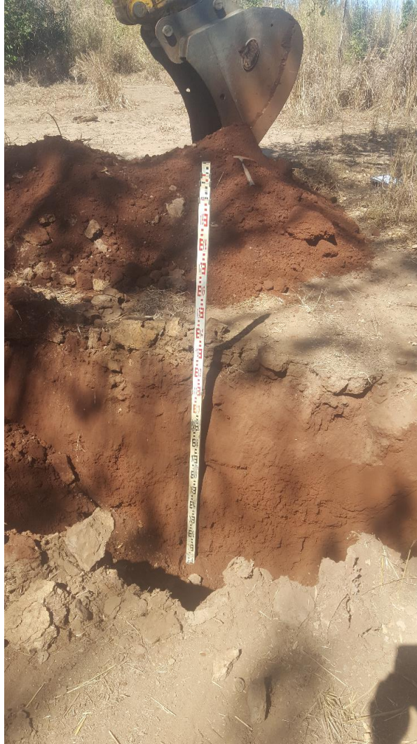
Figure 7. Site 3 test pit excavation for the investigation of radiation levels
